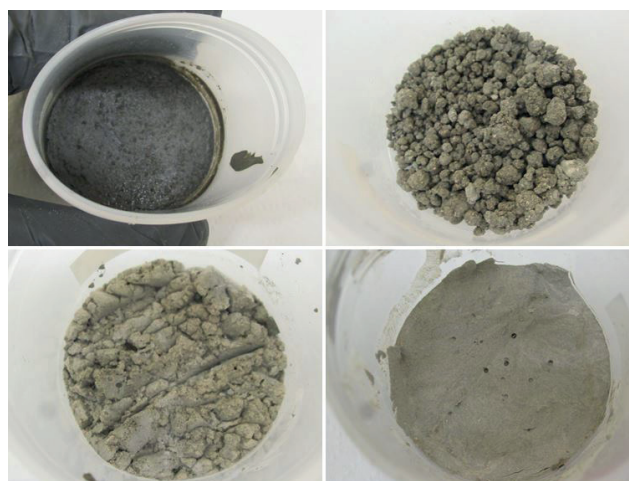
Fig. 2 The stages of the mix design development
