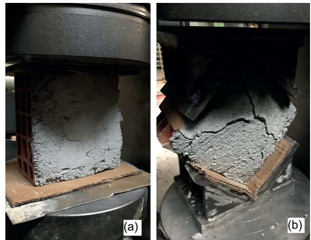
Fig. 4 Orthogonal (a) and diagonal (b) loading of prisms
