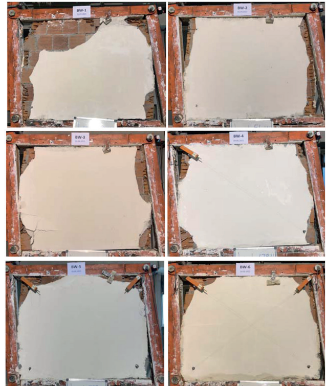
Fig. 7 Failure modes of the reference infill walls
