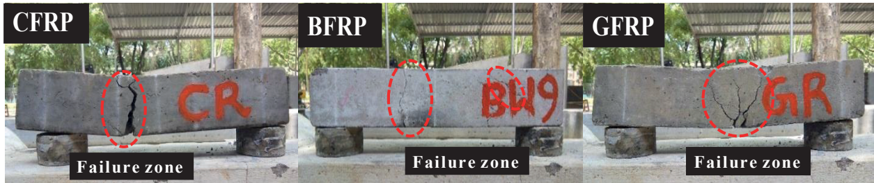
Fig. 9 Typical failure mode of test beams and failure pattern
