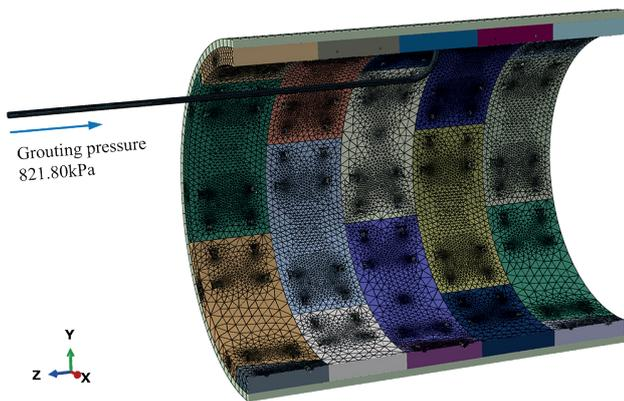
Fig. 6 Model profiles of segments and soil-slurry layers
