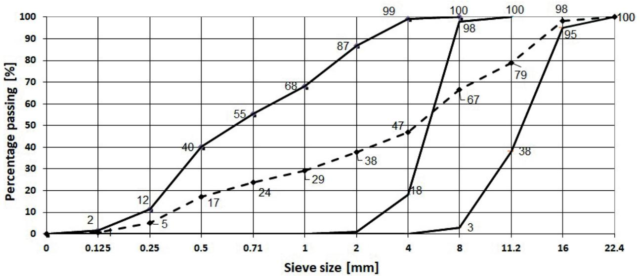
Fig. 2 Particle size distribution of fractions 0/4 mm, 4/8 mm, 8/16 mm and fractions mix of river aggregate
