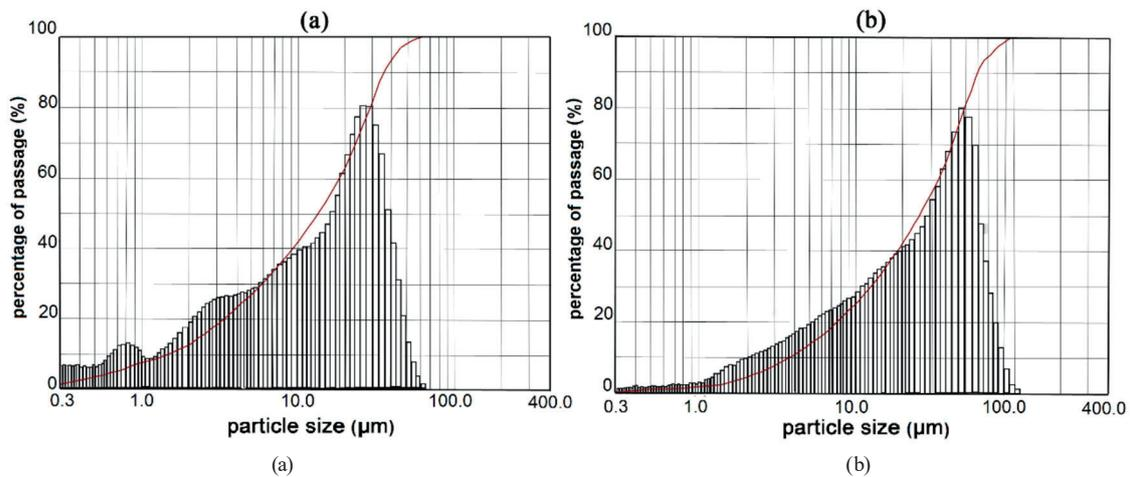
Fig. 1 Particle size distribution of Portland cement CEM I 52.5R (a) and CRT glass (b)
