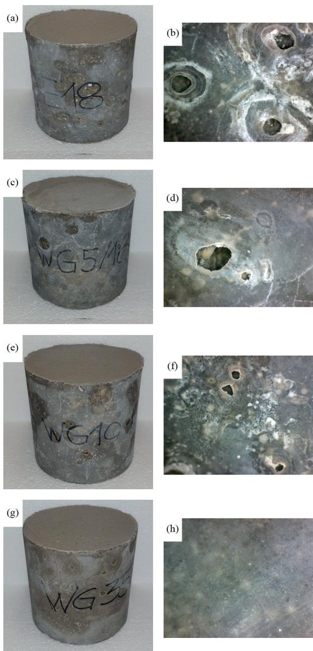
**Fig. 4** Appearance of the sample surface after 36 months of curing in  $\text{Na}_2\text{SO}_4$  – reference concrete E (a) and its magnification (b), WG5 (c) and its magnification (d), WG10 (e) and its magnification (f), WG35 (g) and its magnification (h)
