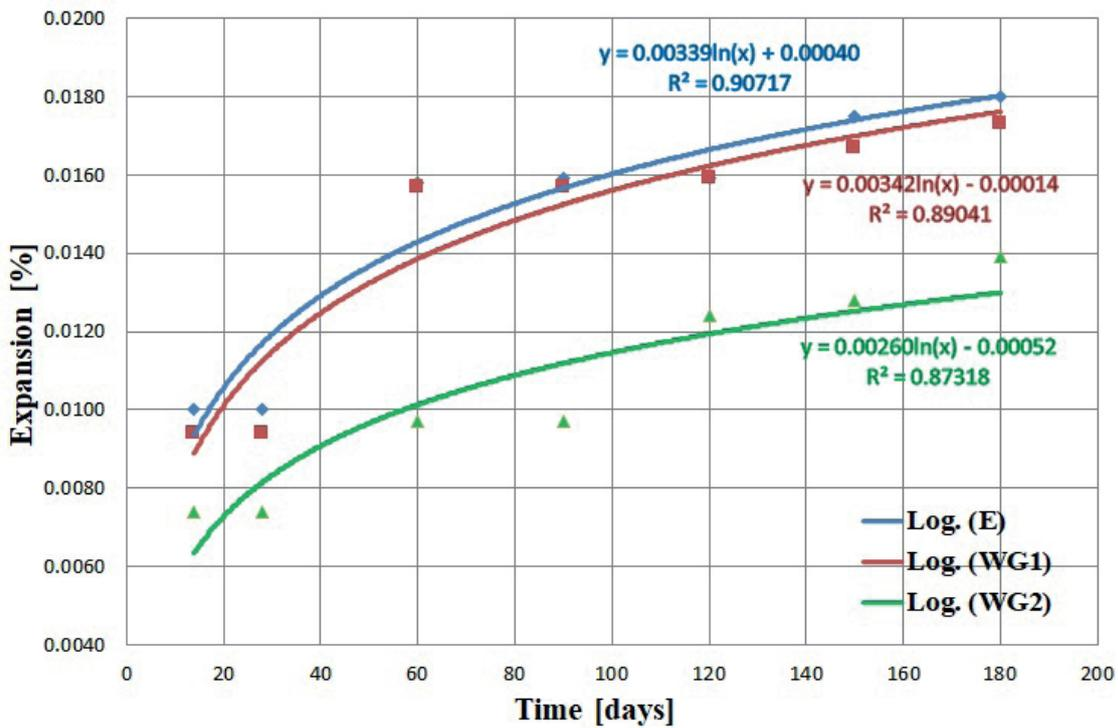
Fig. 3 Expansion of mortar prisms with the addition of CRT glass in the function of time
