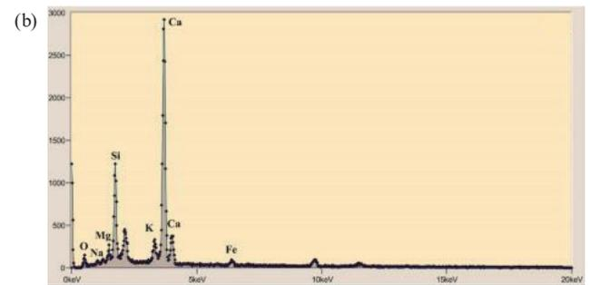
Fig. 6 WG15 concrete 3500× magnification (a); EDS spectroscopy (b)
