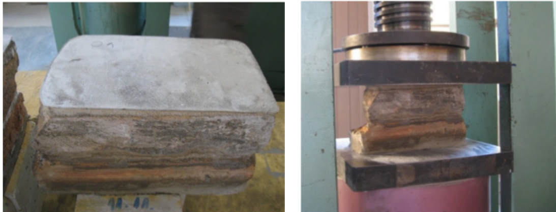
Fig. 7. Testing compressive strength
