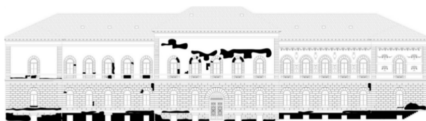
Fig. 5. Damaged segments due to the rising damp process
