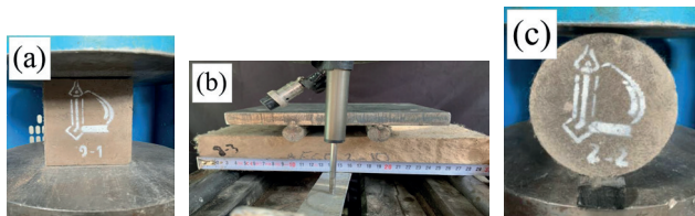
Fig. 7 Specimens under testing: (a) compressive, (b) flexural, and (c) tensile
