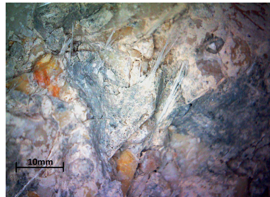
Fig. 6 The internal structure of glass fiber reinforced concrete sample
