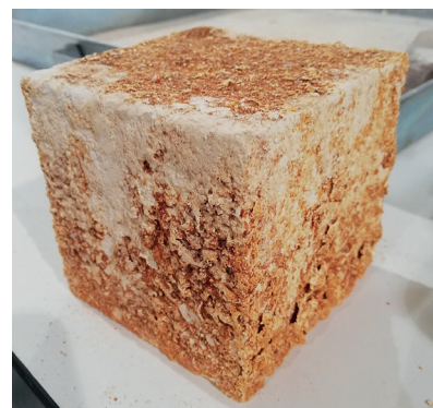
Fig. 10 Acid effect on cubic concrete specimens
