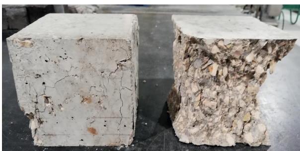
Fig. 3 The appearance of GFRC and control concrete samples after the compressive strength test
