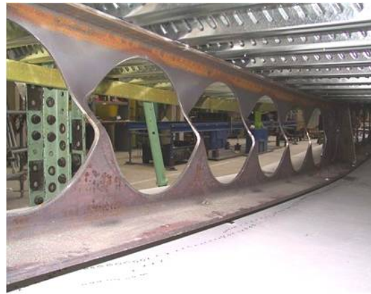
b) Web-post buckling mode
