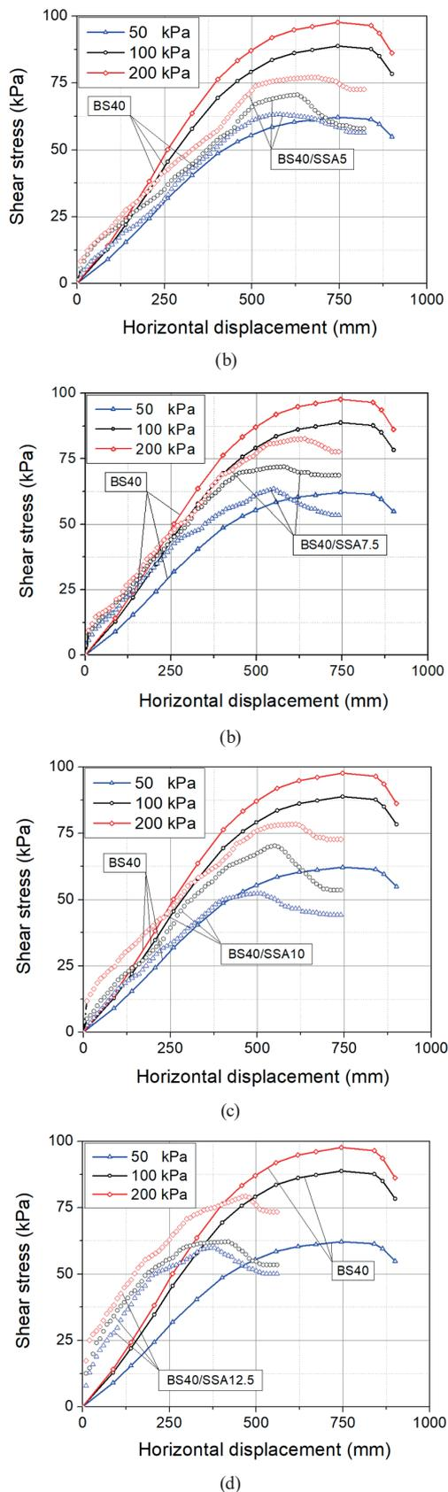
**Fig. 9** Direct shear test results of the BS40 and BS40/SSA mixtures with varied contents of SSA; (a) 5% SSA, (b) 7.5% SSA, (c) 10% SSA, (d) 12.5% SSA
