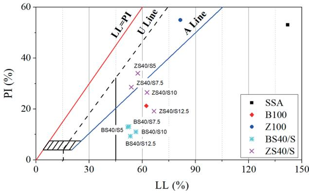
Fig. 14 Consistency limits of the specimens plotted on the Casagrande plasticity chart
