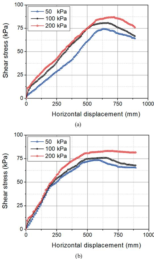
Fig. 7 Direct shear test results of (a) B100 and (b) Z100 specimens
