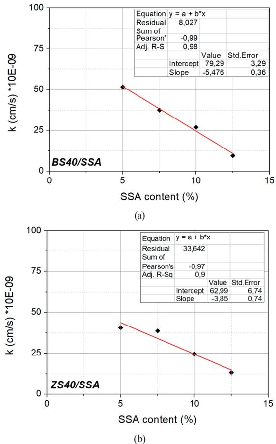
Fig. 16 The variation of the permeability coefficient with SSA content in the mixtures; (a) BS40/SSA, (b) ZS40/SSA specimens
