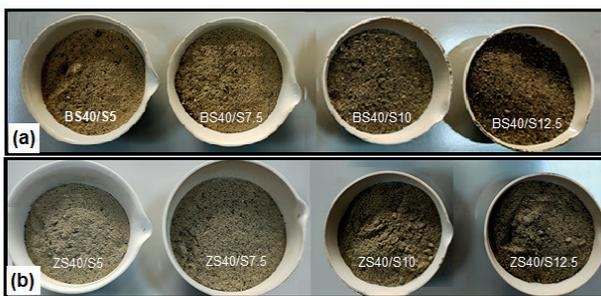
Fig. 4 Materials used in the experiments; (a) bentonite and (b) zeolite mixtures with varied contents of SSA
