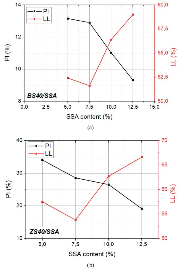
Fig. 13 The variation of the consistency limits with SSA content in the mixtures; (a) BS40/SSA, (b) ZS40/SSA specimens
