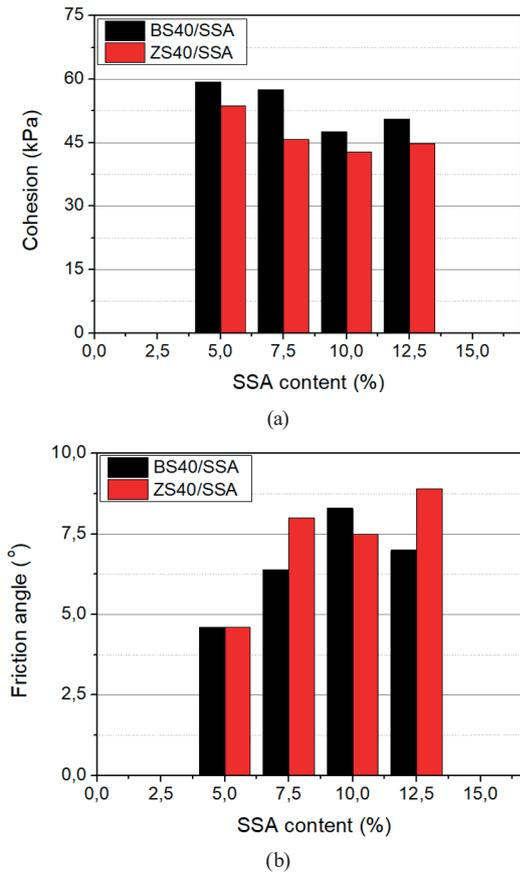
Fig. 12 The variation of (a) cohesion and (b) friction angle with SSA content in the mixtures
