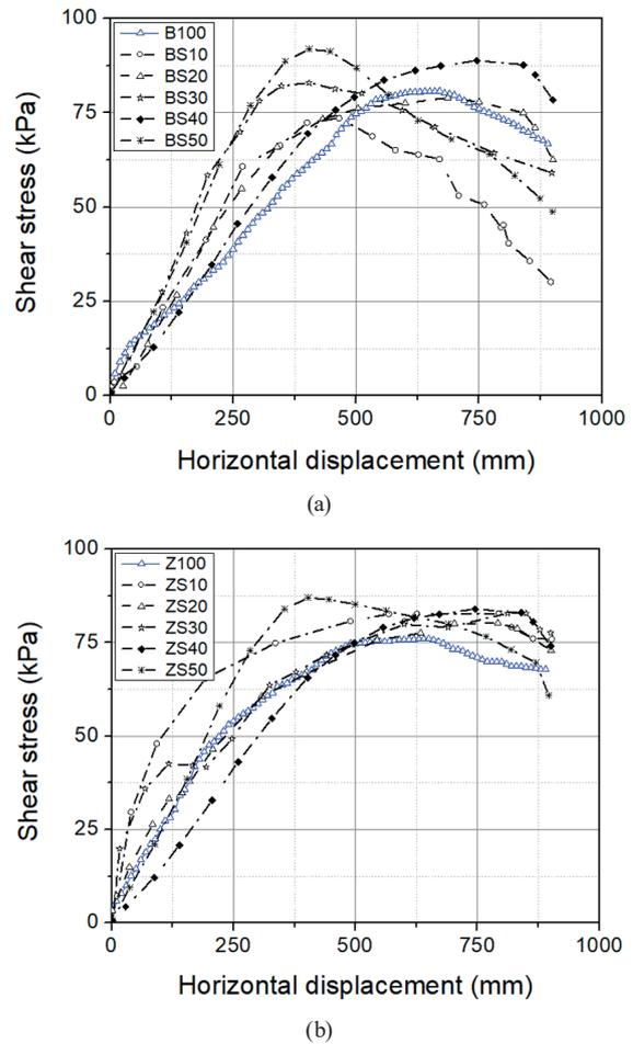
Fig. 8 Direct shear test results of (a) bentonite and (b) zeolite with sand mixtures under 100 kPa normal stress
