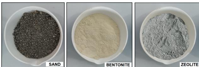
Fig. 3 View of the sand, bentonite and zeolite materials
