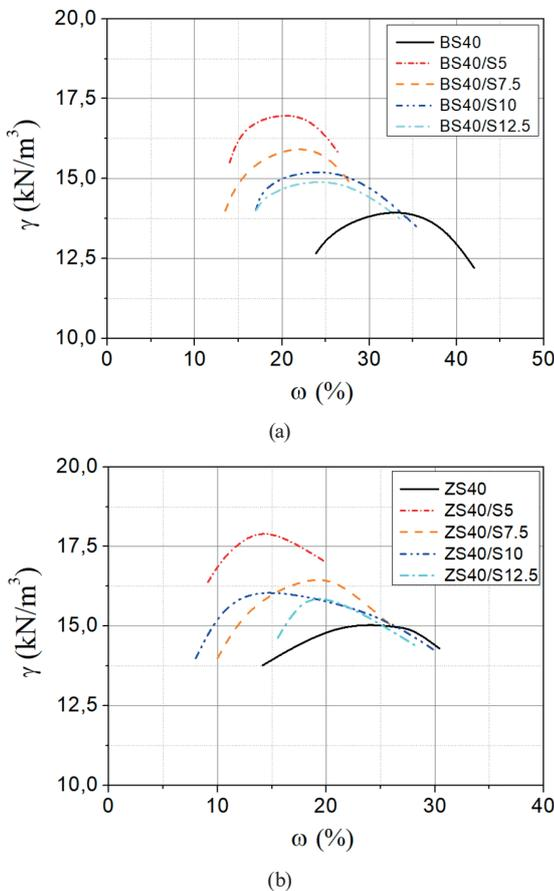
Fig. 15 Compaction curves of (a) BS specimens and (b) ZS specimens
