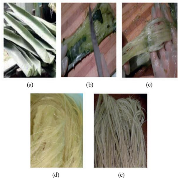
**Fig. 1** Various phases of extraction of *Agave americana*: a) Blades used in fibers extraction, b) Crushing of the fibers, c) Extraction fibers, d) *Agave americana* fibers before drying, e) *Agave americana* fibers after drying
