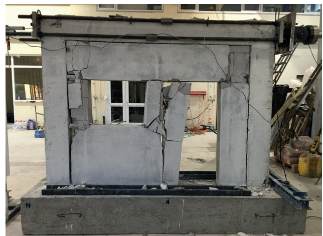
Fig. 28 (a) Crack map, (b) Failure pattern of RCF-5
