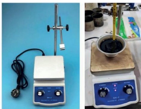
Fig. 2 Hot plate magnetic stirrer device
