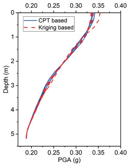
Fig. 4 PGA for CPT-based and Kriging-based site profile
