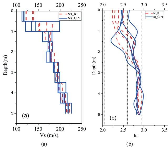
Fig. 3 Shear wave velocity profile (a) and Soil behaviour type index profile (b)
