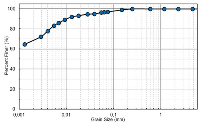
**Fig. 1** Particle size distribution of the clay soil
