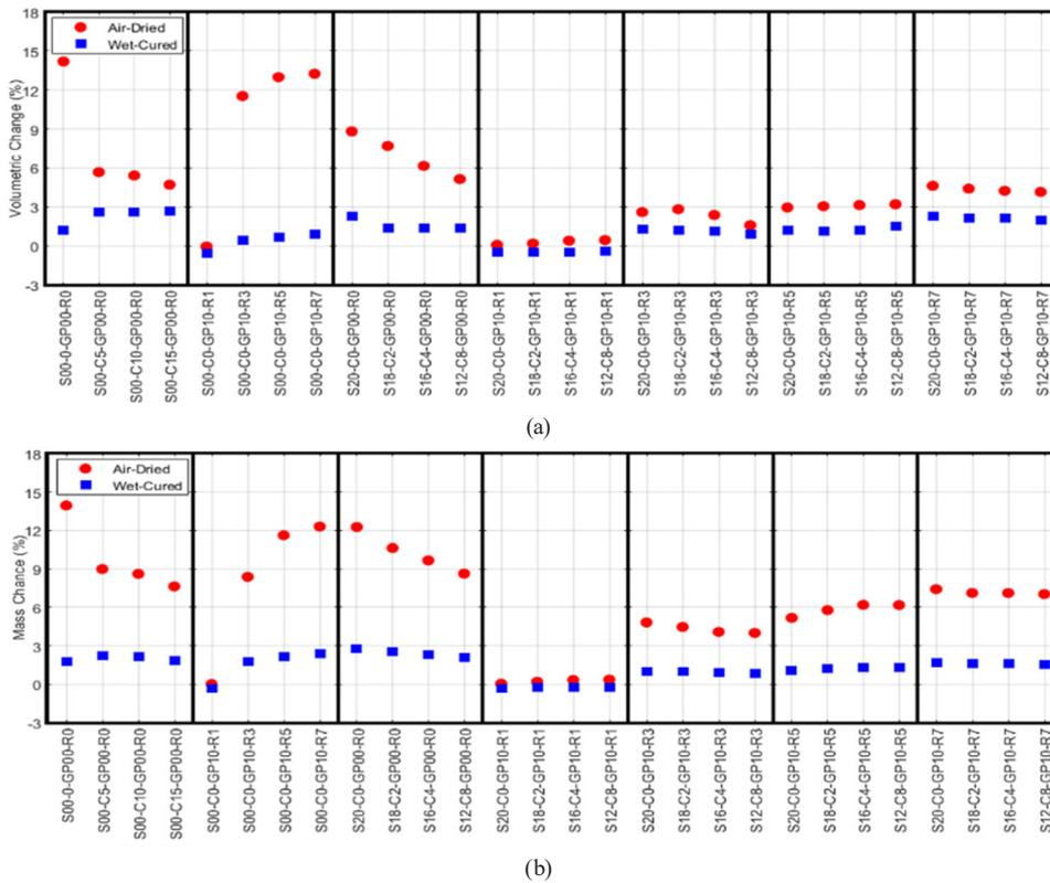
**Fig. 8** In air-dried and wet-cured conditions, 90 days volumetric and mass percentage change of untreated clay and stabilized soils; (a) Percentage of volumetric change, (b) Percentage of mass change
