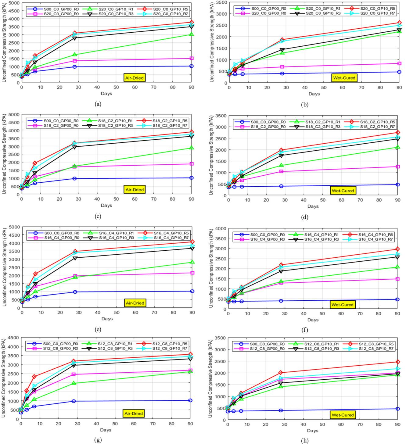
**Fig. 5** Time-dependent compressive strength development of untreated and treated clay samples under air-dried and wet-cured conditions; (a–b) GGBS 20 wt%, OPC 0 wt%, and alkali activator 10 wt% of the clay, (c–d) GGBS 18 wt%, OPC 2 wt%, and alkali activator 10 wt% of the clay, (e–f) GGBS 16 wt%, OPC 4 wt%, and alkali activator 10 wt% of the clay, (g–h) GGBS 12 wt%, OPC 8 wt% and alkali activator 10 wt% of the clay
