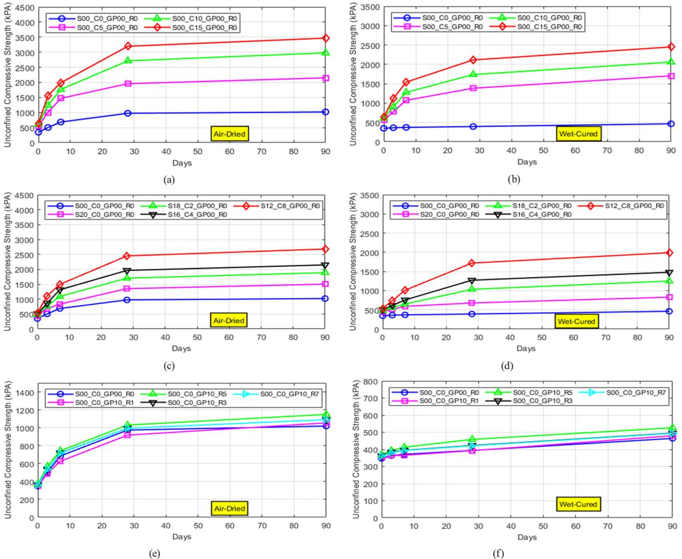
**Fig. 2** Time-dependent compressive strength development of untreated and treated clay samples under air-dried and wet-cured conditions; (a-b) OPC, (c-d) binary GGBS + OPC mix, and (e-f) only alkali activator
