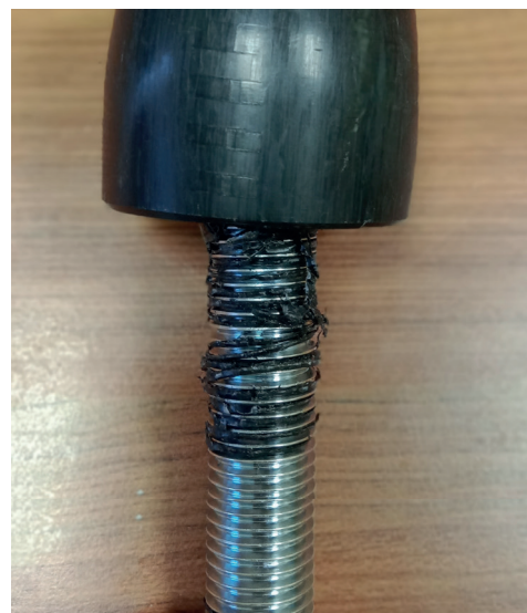
Fig. 4 Polyamide nut slide on bolts
