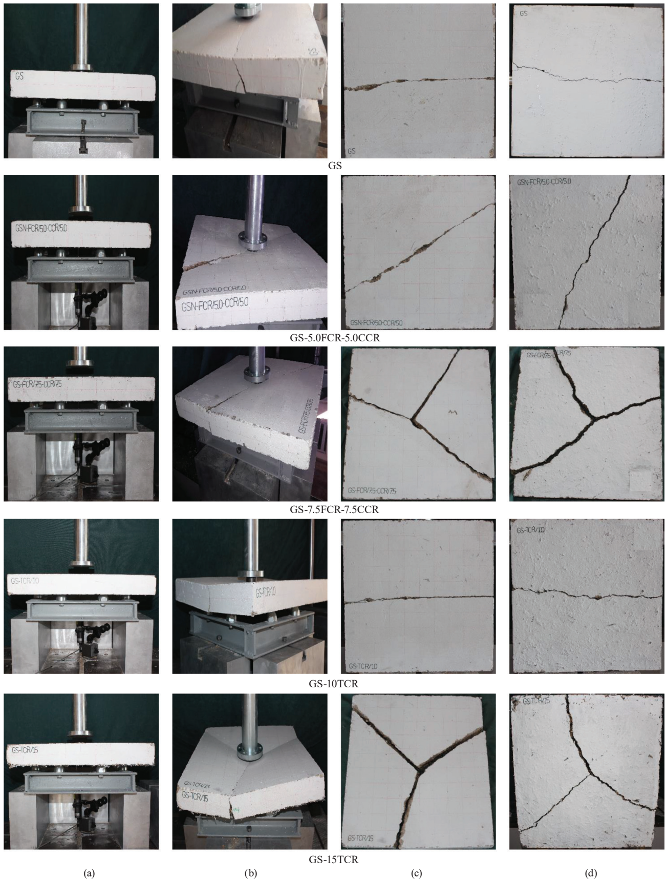
Fig. 6 Failure modes of AAC slabs after punching shear tests; (a) Before failure, (b) After failure, (c) Front surface after failure, (d) Back surface after failure
