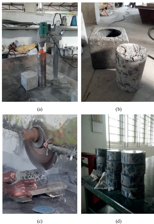
Fig. 5 Making of sample for sorptivity test (a) Drilling of concrete cubes, (b) Drilled concrete cubes, (c) Cutting of concrete cylinder, (d) Sample for sorptivity test
