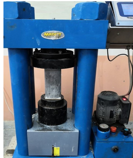
Fig. 5 Testing of control specimens for compressive strength
