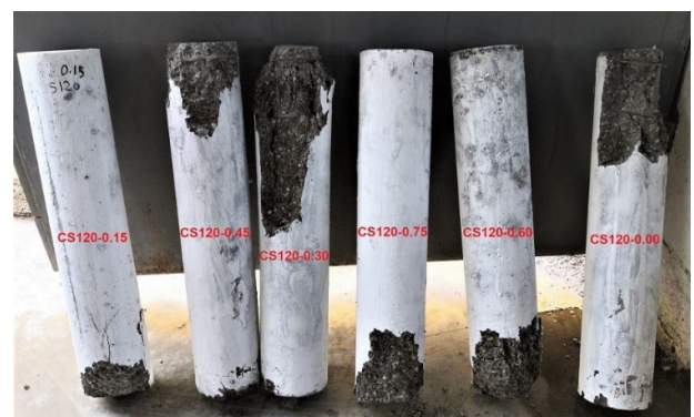
Fig. 8 Failure patterns of short columns
