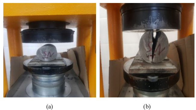
Fig. 9 Split tensile strength tests, (a) Before test, (b) After test
