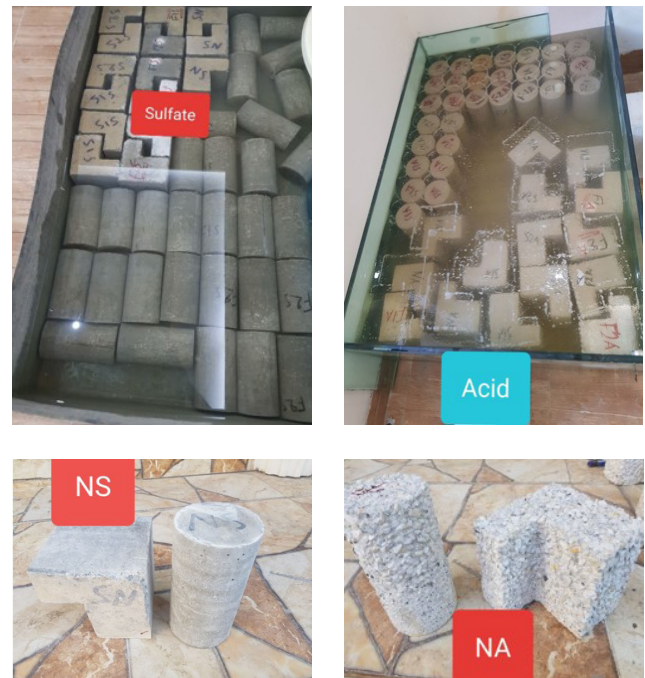
Fig. 2 Sample exposure to MgSO 4 and H 2 SO 4 and condition after 1 month exposure
