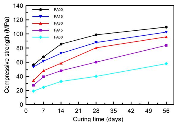
Fig. 7 Effect of FA content on compressive strength
