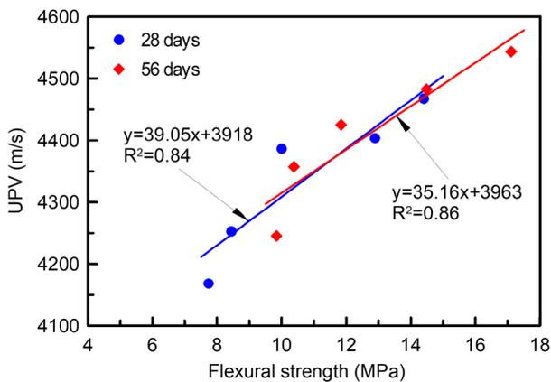
Fig. 14 Correlation between UPV and flexural strength
