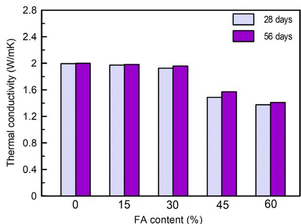
Fig. 18 Effect of FA content on thermal conductivity
