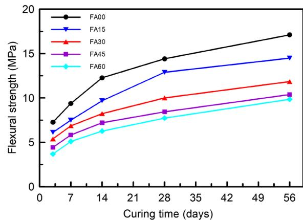
Fig. 8 Effect of FA content on flexural strength
