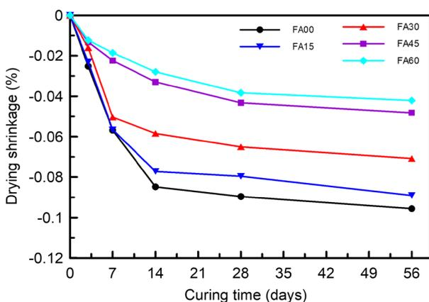
Fig. 17 Effect of FA content on drying shrinkage
