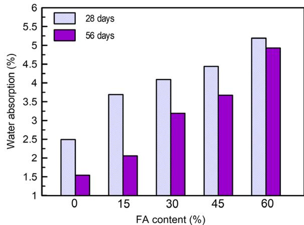
Fig. 15 Effect of FA content on water absorption
