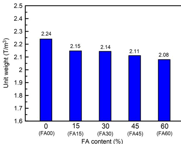
Fig. 6 Effect of FA content on unit weight
