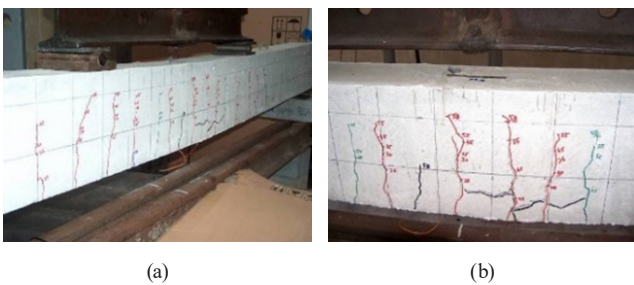
Fig. 10 Crack distribution at beam B-G3 (bypassing 20∅): (a) general view, (b) detail view
