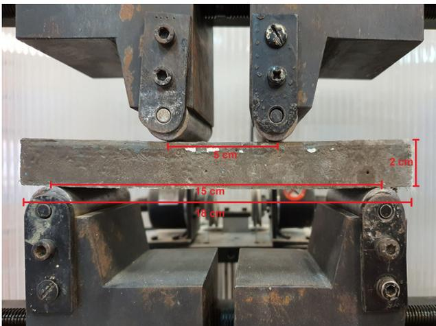
Fig. 5 The four-point bending setup
