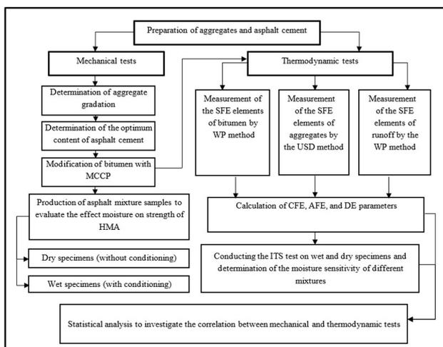
Fig. 1 The test design algorithm
