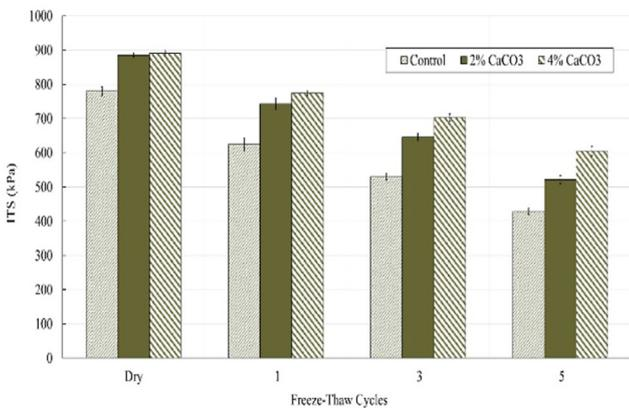
Fig. 6 Results of the ITS test on the modified HMA containing limestone aggregates
