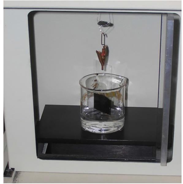
**Fig. 5** Immersing the asphalt-coated surface and removing it in the WP
