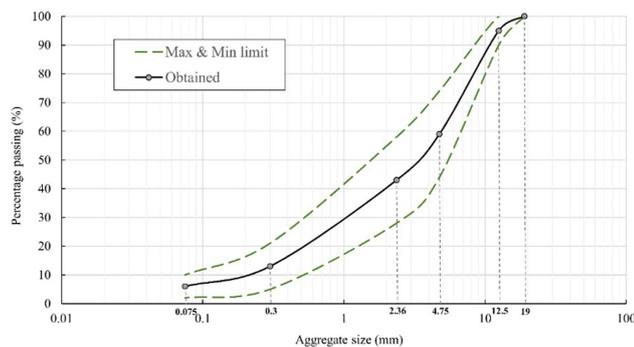
**Fig. 2** The size distribution of used aggregates
