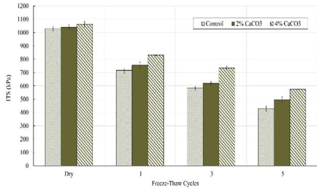
Fig. 8 Results of the ITS test on the modified HMA containing quartzite aggregates
