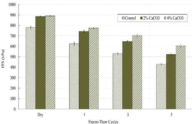
Fig. 7 Results of the ITS test on the modified HMA containing granite aggregates
