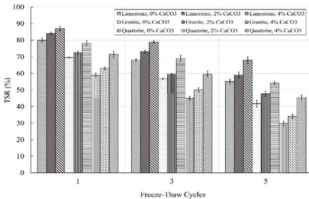
Fig. 9 TSR parameters of different HMA samples
