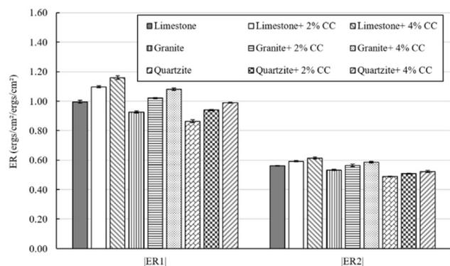
Fig. 10  $ER_1$  and  $ER_2$  bond energy parameters of different HMA
