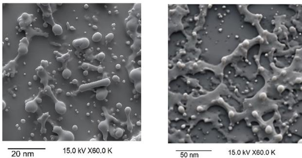
**Fig. 3** The distribution of MCCP in bitumen
