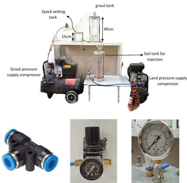
**Fig. 2** Injection simulation device
