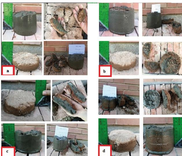
Fig. 4 The injected area in the form of a cylinder for various grout pressure (a) 1.5 bar, (b) 2 bar, (c) 2.5 bar, (d) 3 bar
