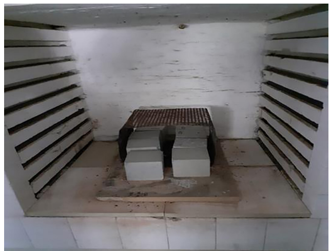
Fig. 3 Concrete samples in the electric oven
