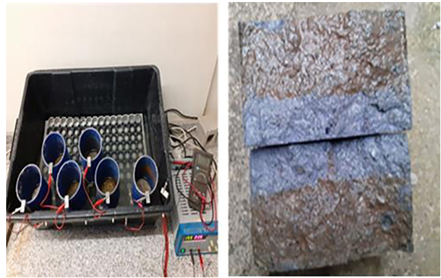
Fig. 2 Image of sample preparation for chloride penetration resistance test
