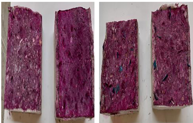
Fig. 4 Spray samples with phenolphthalein to determine carbonation depth
