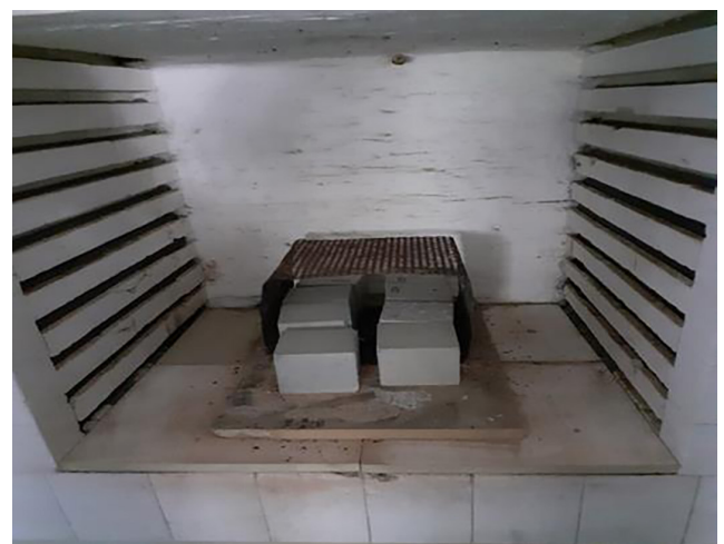
Fig. 3 Concrete samples in the electric oven
