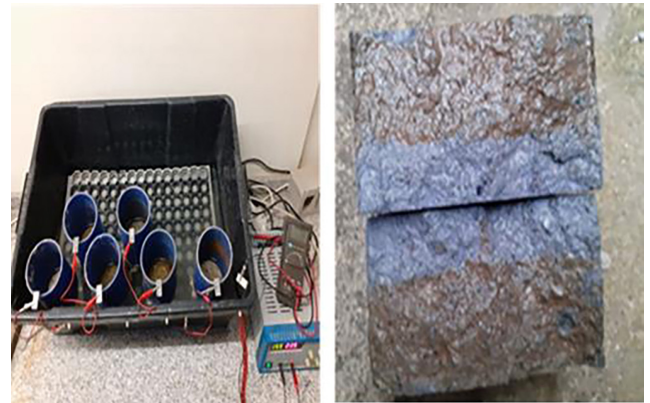
Fig. 2 Image of sample preparation for chloride penetration resistance test
