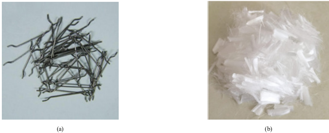
Fig. 2 Steel and polypropylene fibers used in experimental samples (a) steel fibers and (b) polypropylene fibers
