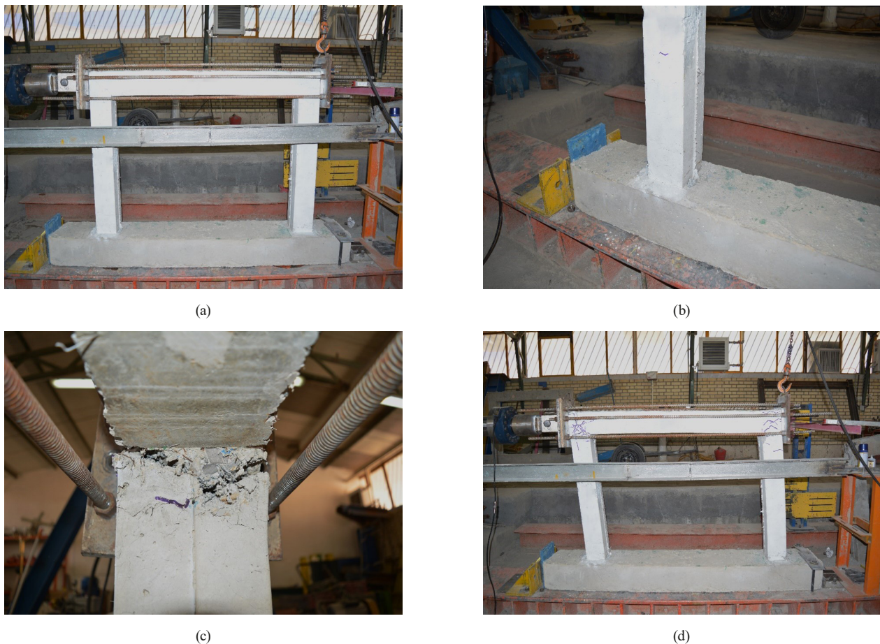
Fig. 9 Images related to the test of RCMRF-SF-AEA sample (a) at the beginning of the test (b) column foot connection at 4% drift (c) beam to column connection at the end of test (d) end of the test
