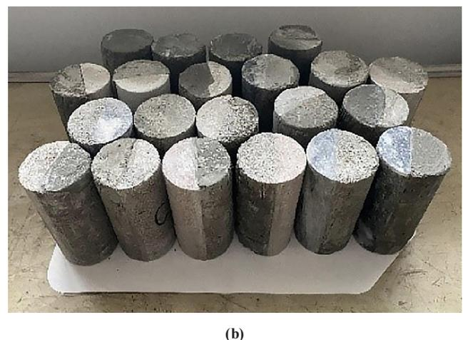
Fig. 2 Process and finished product of rock-concrete composite sample
