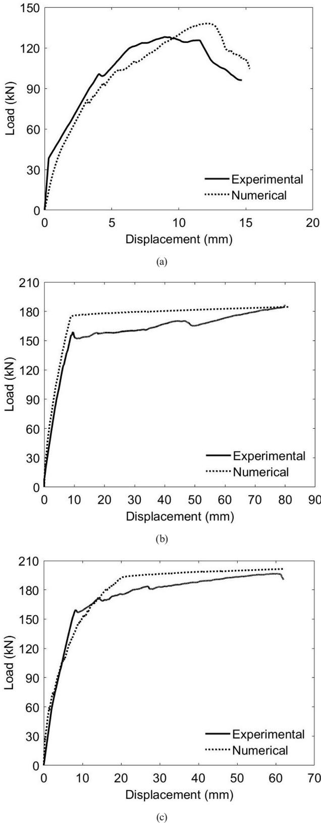
Fig. 10 Comparison between the experimental and numerical results: (a) Specimen BN, (b) Specimen BGS, (c) Specimen BGC
