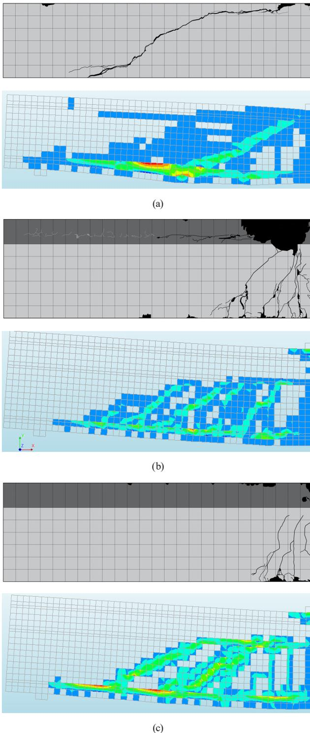
**Fig. 11** Tensile equivalent plastic strains of the test beams:
