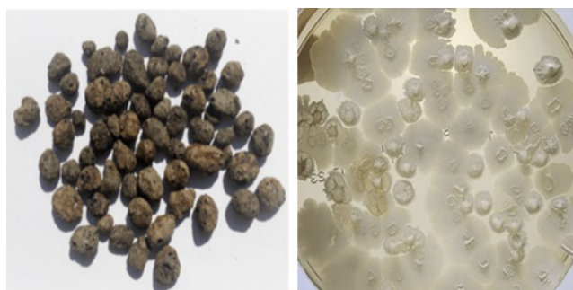
Fig. 4 Light weight aggregate and Bacillus subtilis dispersion
