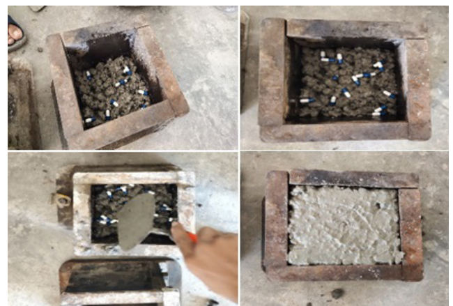
Fig. 3 Encapsulation of silica gels and concrete embedment
