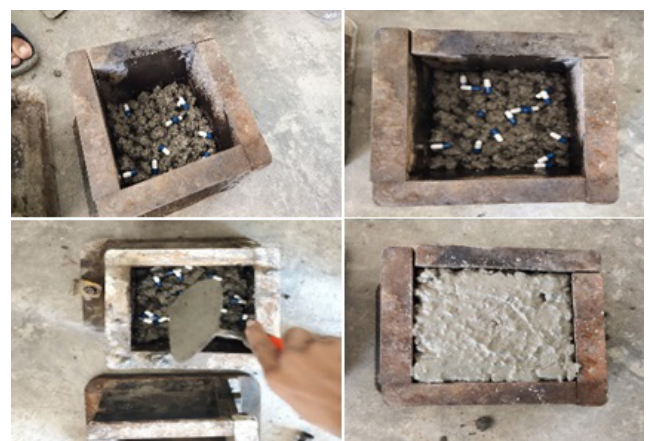
Fig. 3 Encapsulation of silica gels and concrete embedment
