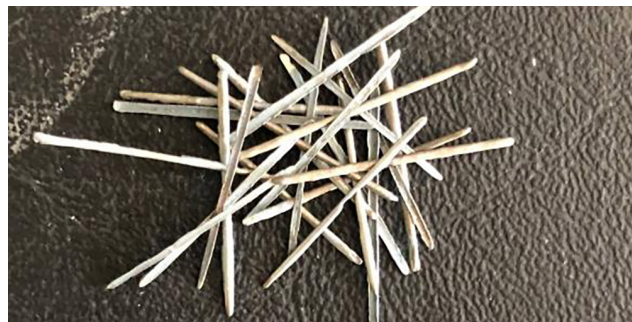
Fig. 1 Straight steel micro-fibers
