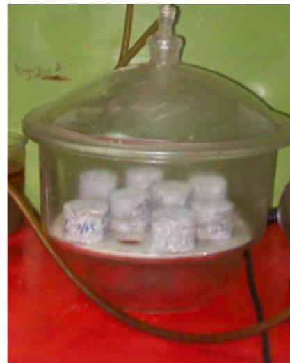
Fig. 8 Vacuum saturation equipment
