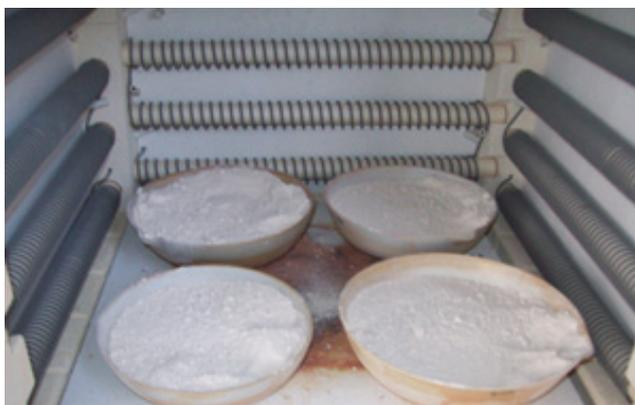
**Fig. 3** Calcination of kaolin in the furnace
