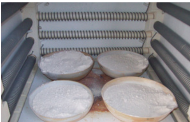
Fig. 3 Calcination of kaolin in the furnace
