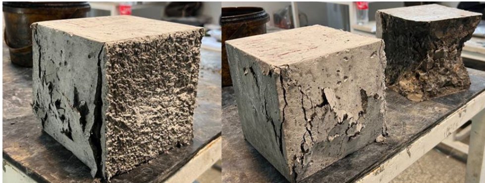
Fig. 4 Compressive strength test of cubic specimens
