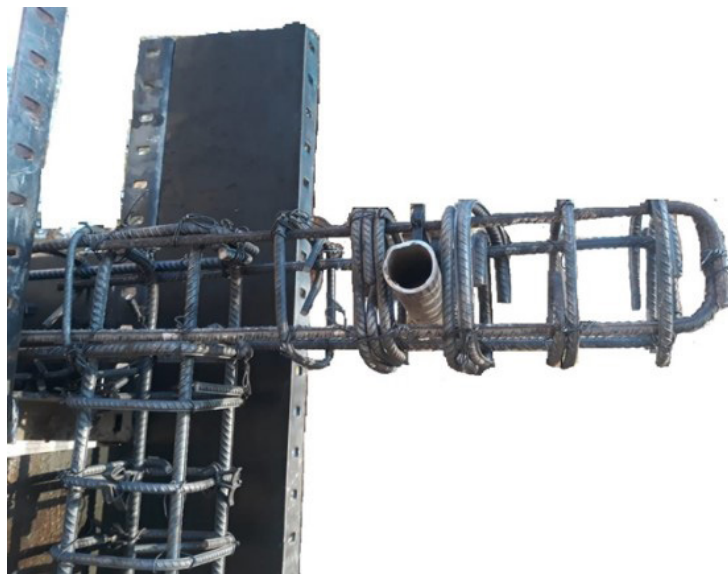
Fig. 8 Using a doubled stirrup in the console connected to the concrete frame (cyclic load application area)
