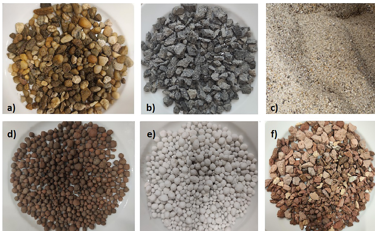
Fig. 1 Aggregates used in the research, (a) River quartz aggregates, (b) Crushed andesite, (c) Quartz sand, (d) Expanded clay, (e) Expanded glass, and (f) Crushed clay bricks
