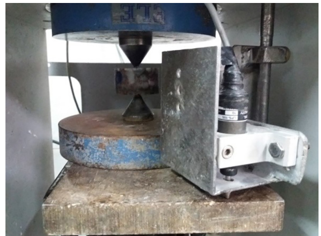
Fig. 10 Installing the strain gauge on the metal plate located on the loading platform below the samples
