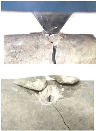
Fig. 11 Local failure during point load tests
