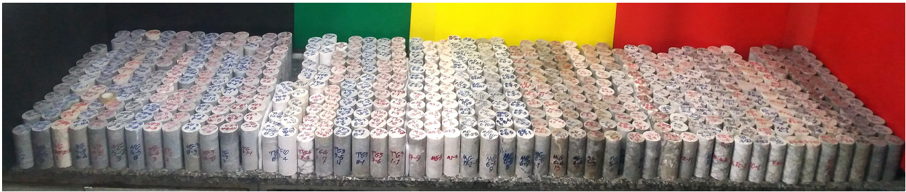
Fig. 2 Rows of red, yellow, green and black, respectively, several rock core samples of the Konjun-Cham, Meymeh, Kangir and Nargesi dam sites
