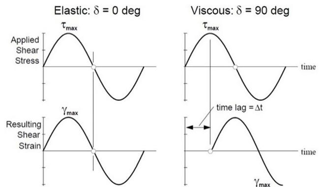
Fig. 6 Schematic representation of the applied stress and the resulting strain
