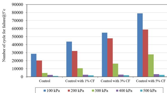
Fig. 11 Number of cycles for failure at 5 °C at different levels of stress
