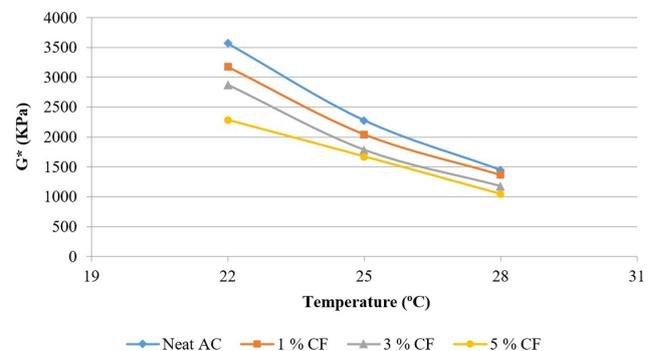
Fig. 9 Complex modulus values in control and modified asphalt binders
