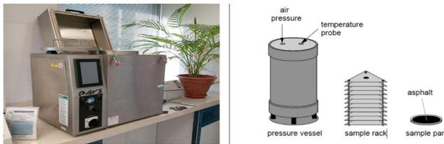
Fig. 4 Overall and schematic view of the PAV device
