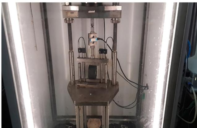
Fig. 7 The loading process of ITFT
