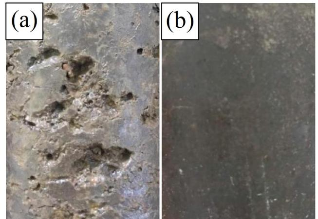
Fig. 8 Surface comparison: (a) Etching pits on the surface of specimens added with 0.3% soluble sodium salts; (b) the surface of B2 specimens and specimens added with B2 and 0.3%  $\text{CaCl}_2$
