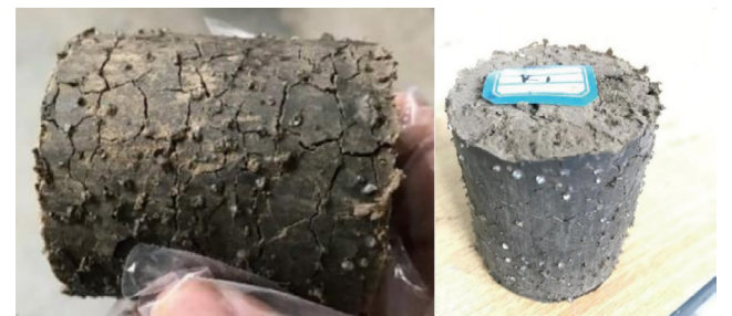
Fig. 11 Specimens cracking with a dosage of 0.2% CPAM by dry mixing
