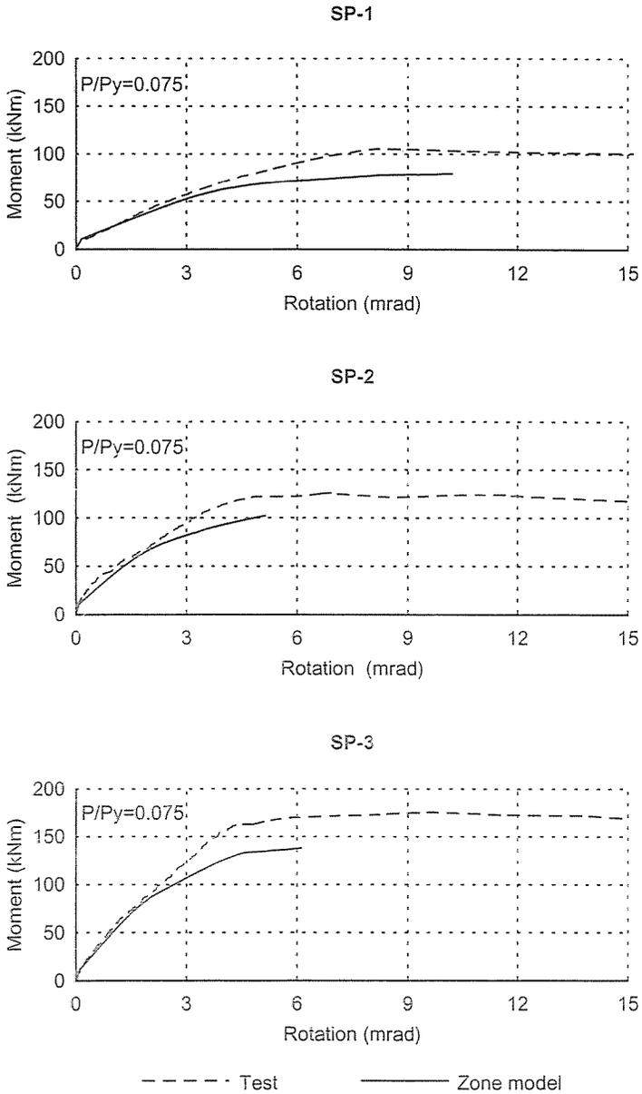
Fig. 9. Experimental and calculated moment-rotation curves
