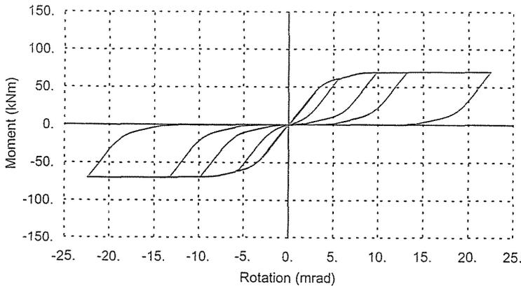
*Fig. 11.* Calculated cyclic moment-rotation curve of SP-1
