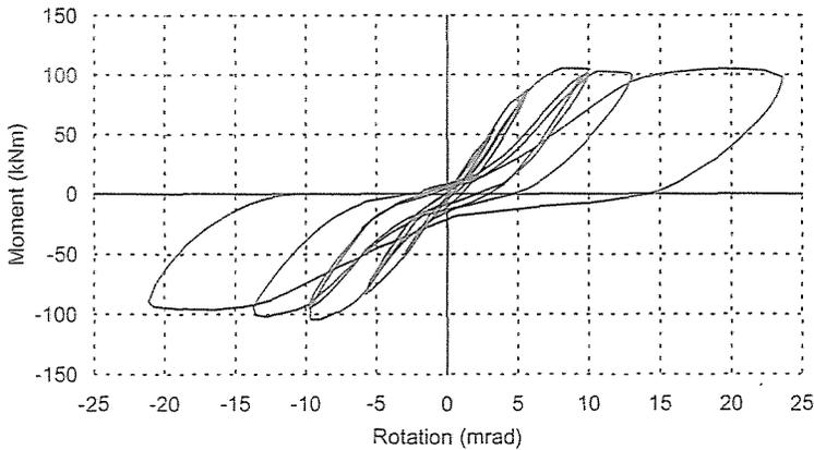
*Fig. 10.* Experimental cyclic moment-rotation curve of SP-1
