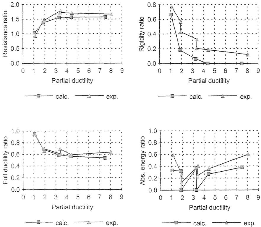
Fig. 13. Characterizing parameters of the moment-rotation curves of SP-1
