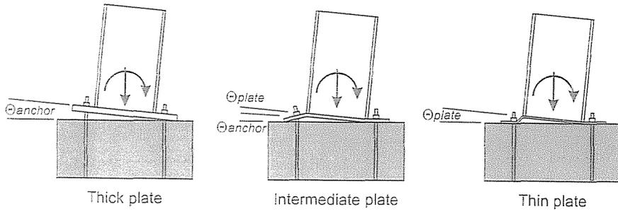
Fig. 4. Classification of mixed connections (ASTANEH et al., 1992)
