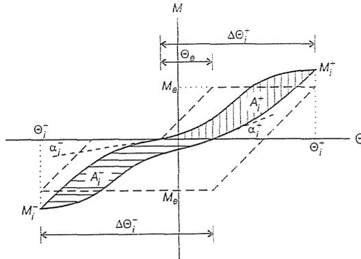
Fig. 12. Interpretation of the characterizing parameters of cyclic curves
