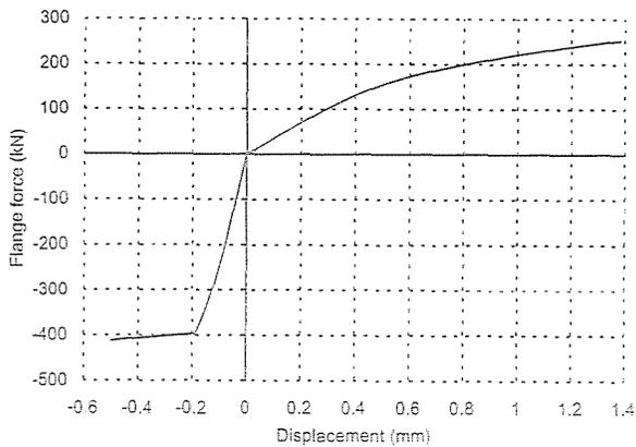
Fig. 8 Calculated flange force – displacement relationship of SP-2
