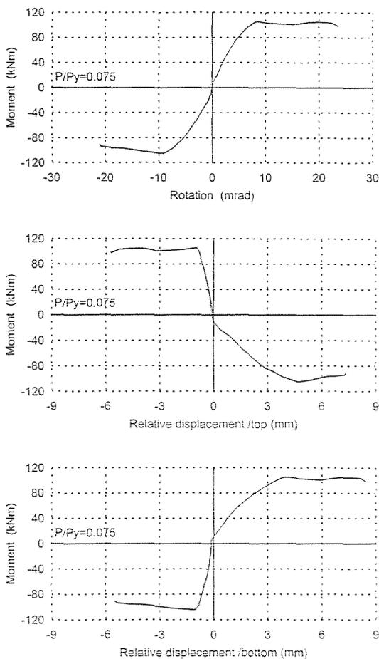
Fig. 3. Moment – rotation and moment – relative displacement curves of SP-1
