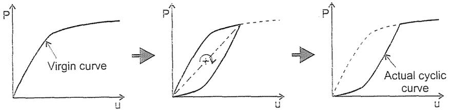
Fig. 7. Derivation of cyclic  $P - u$  curve
