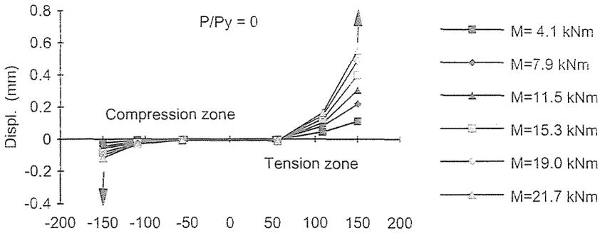
Fig. 5. End-plate deformation of SP-1
