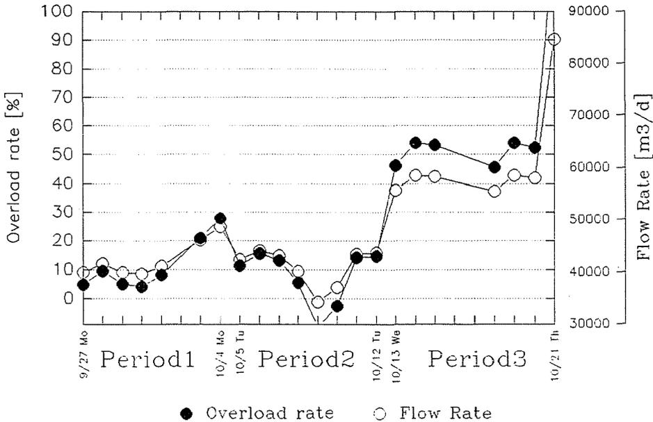
Fig. 2. Overload rate (compared to 1993 average) and flow rate for the experimental train
