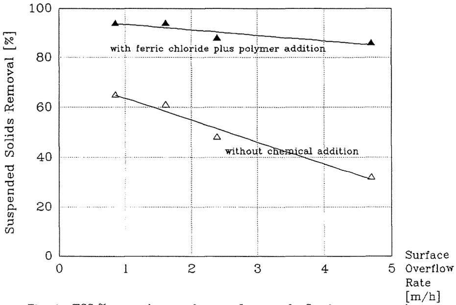
Fig. 1a. TSS % removal vs. surface overflow rate for Sarnia treatment plant
