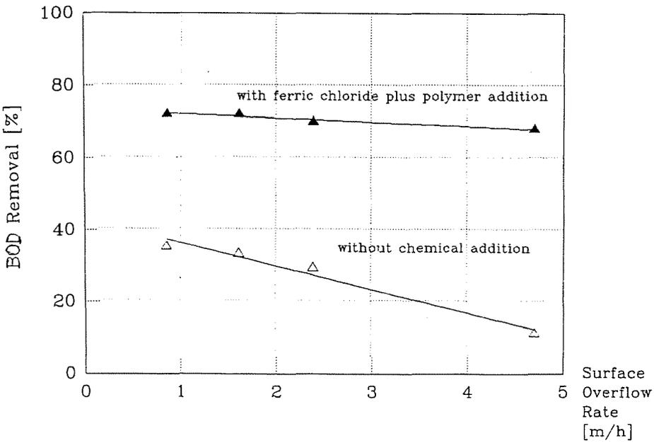
Fig. 1b. BOD % removal vs. surface overflow rate for Sarnia treatment plant
