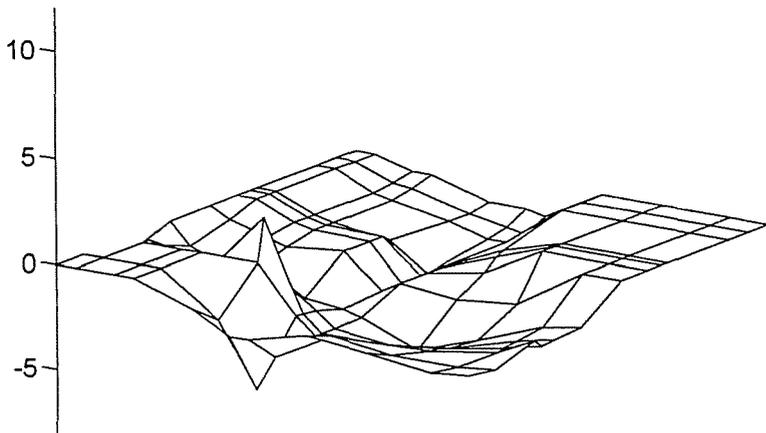
Fig. 4. The scenography of the values of foundation body movements and deformations determined at the 1. and 2. testing measurements of the Budapest-City-Shopping-Business-Centre
