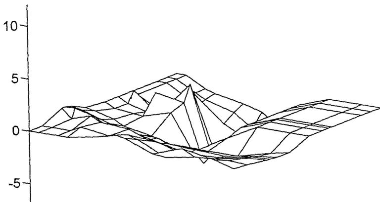
Fig. 2. The scenography of the values of foundation body movements and deformations determined at the 1. testing measurement of the Budapest-City-Shopping-Business-Centre
