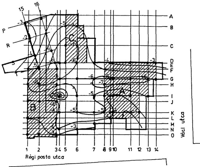
Fig. 5. The values of foundation body movements and deformations given in elevation numbers, determined at the 4. testing measurement of the Budapest-City-Shopping-Business-Centre as well as the presentation of their lines of levels
