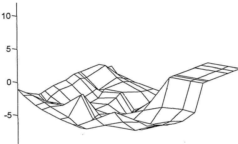
Fig. 6. The scenography of the values of foundation body movements and deformations determined at the 4. testing measurement of the Budapest-City-Shopping-Business-Centre as well as the presentation of their lines of levels
