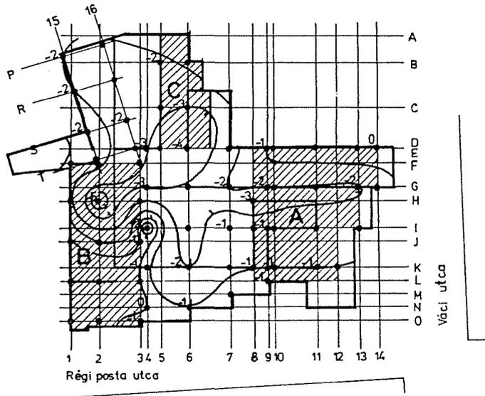
Fig. 3. The values of foundation body movements and deformations given in elevation numbers, determined at the 2. testing measurements of the Budapest-City-Shopping-Business-Centre as well as the presentation of their lines of levels
