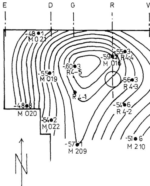
Fig. 8. The displacement values of the testing points of foundation body given in elevation numbers at the IV. block of the Nuclear Power Station in Paks as well as the presentation of their lines of levels
