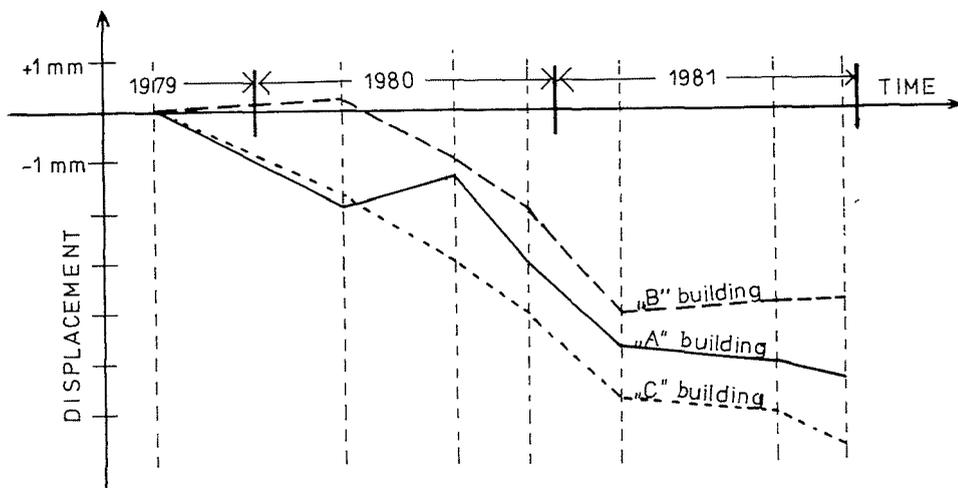
Fig. 7. Average displacements of the testing points at the building parts of the Budapest-City-Shopping-Business-Centre in function of time
