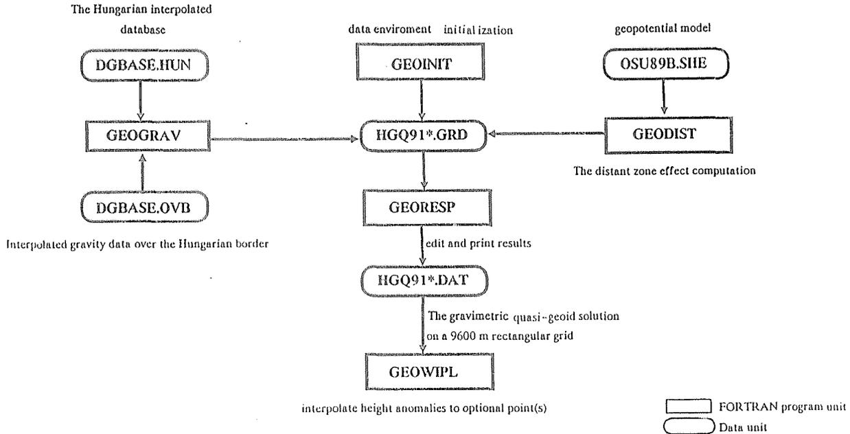
Fig. 5. Simplified flowchart of the GEOMETR program system without parts for astro-gravimetric geoid determination.
