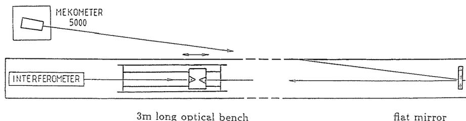
Fig. 6. The layout of the calibration setup
