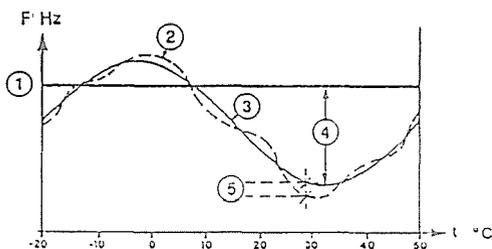
*Fig. 7.* The temperature-frequency correction function
