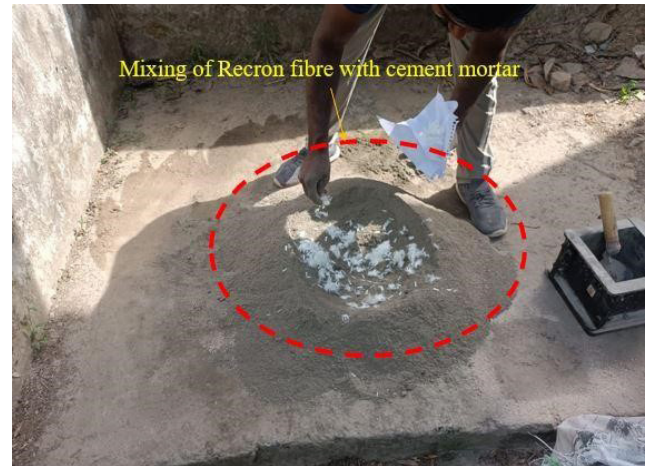
Fig. 1 Mixing of cement mortar with Recron fibers
