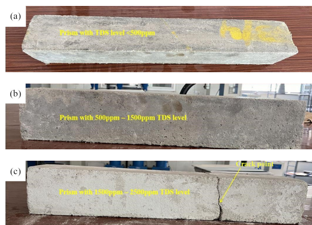
Fig. 8 Prism with various TDS levels (a) <500 ppm (b) 500–1500 ppm (c) 1500–2500 ppm
