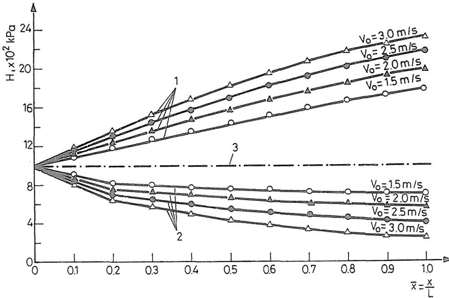
Fig. 4. Extremal pressure variations along pipeline depending on flow velocity:
