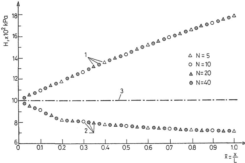
Fig. 5. Extremal pressure variations along pipeline depending on number of scanning sections:
