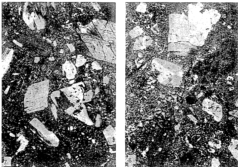
Fig. 7. Biotite-amphibole andezite. Crossed Nikols. Magn.: 27.5 \times Essential minerals: plagioclase, basaltic amphibole, biotite. Porphyric minerals are healthy, sericitized, chloritized. In the embedding material magnetite, quartz, chlorite are present. The amphibole minerals have particle sizes of 1000-2000 \mu\text{m}
