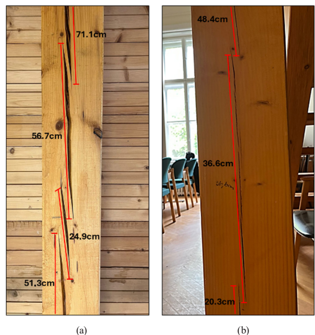
Fig. 1 Crack length measurements on wooden pillars: (a) distribution and extent of surface cracks on Wooden Pillar 1; (b) distribution and extent of surface cracks on Wooden Pillar 3
