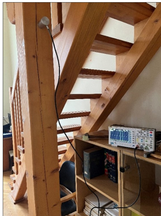
Fig. 2 Ultrasonic testing of the wooden pillar using FNIRSI 1014D digital oscilloscope
